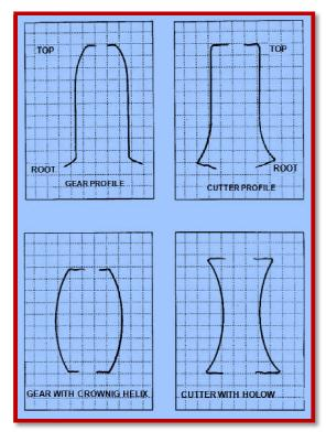
Fig.N 3- Schematics for the gear profile and helix modification and corresponding cutter profile and helix correction
