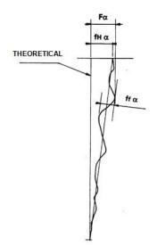
Fig.N°5- Profile error definition
