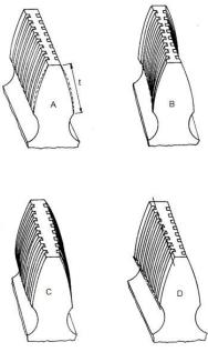
Fig.N°4- Examples of special profiles and helix
